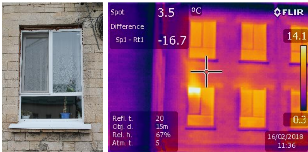
Photo 4 Window of the central façade and it's visualization under the infrared camera
