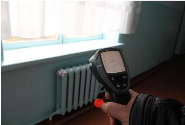
Photo 4 Radiator in the corridor of the first floor and measuring of its temperature.
