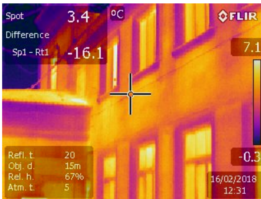
Photo 3 West façade (picture from the infrared camera)
